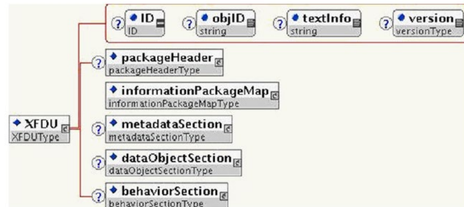
図2: First-Level Decomposition of XFDU Type
