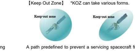
ApproachingA path predefined to prevent a servicing spacecraft from colliding<br/>path:path:with a target upon making an intentional entry into KOZ to approach<br/>the target. An approaching path must not interfere with a protected<br/>area (an area involving the risk of collision) in light of the structure<br/>of a target.
