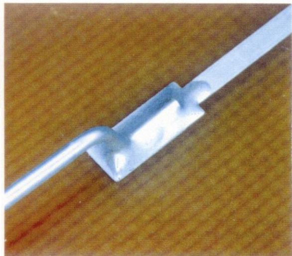
Figure II-4: PWB lapped termination; Round lead (Lead terminated on rectangular pad on same side as part)
