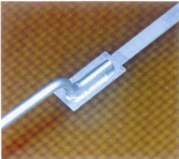
Figure II-4: PWB lapped termination; Round lead (Lead terminated on rectangular pad on same side as part)
