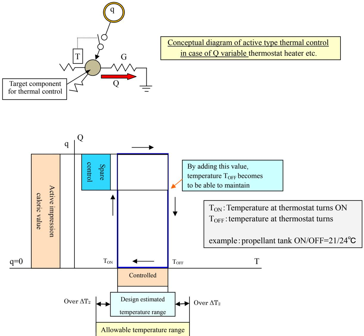
Fig. 5.2.3 Conceptual diagram and design margin of active type thermal control (Q is variable)
