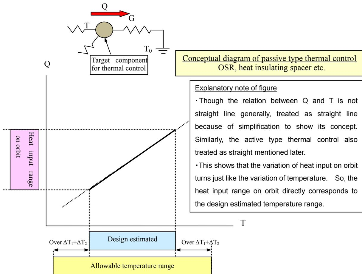
Fig 5.2.1 Conceptual diagram and design margin of passive type thermal control
