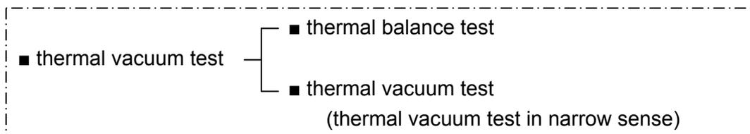
The standard regarding the thermal vacuum test of spacecraft shall follow 2.1 (3) “JERG-2-002 Standard of General Tests for Spacecrafts”, to establish the thermal control design standard, while the thermal balance test is performed for the purpose of validating the thermal control system.
