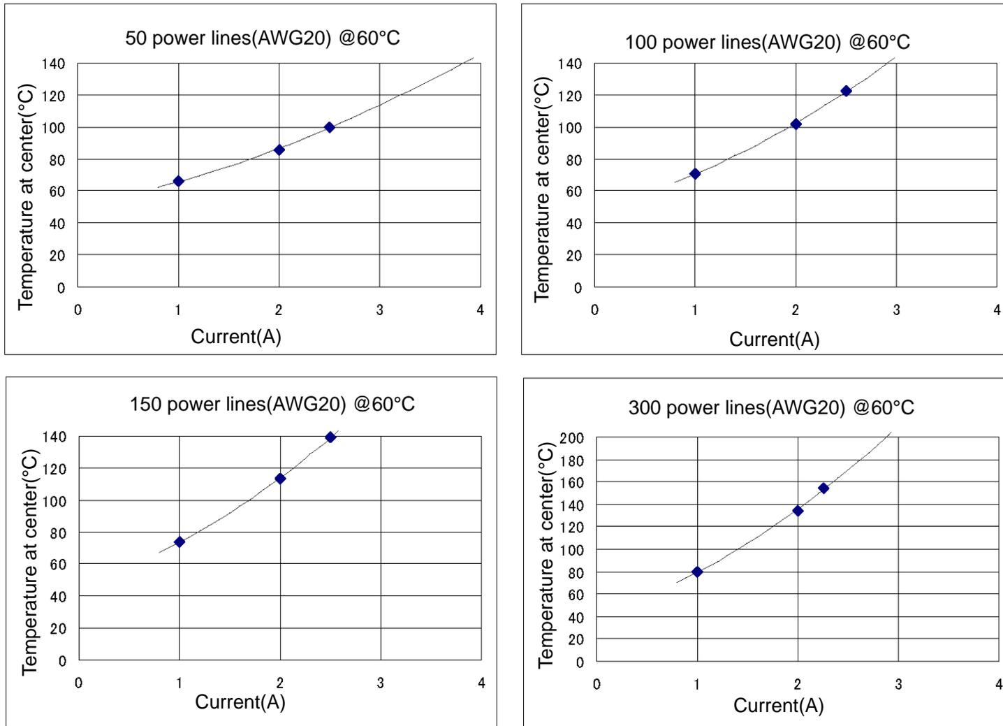
Figure II-2 Results of derating acquisition test conducted on bundled power lines only at an ambient temperature of 60°C
