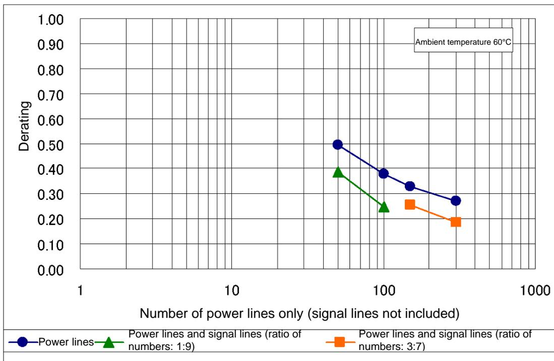
Figure 5.2-2 Derating of maximum current in single line with number of wire bundles as parameter (ambient temperature: 60°C)
